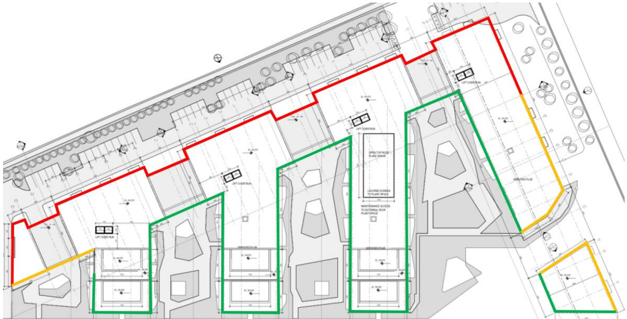
Figure 10.11 Façade Noise Levels (see Table 10.17)
